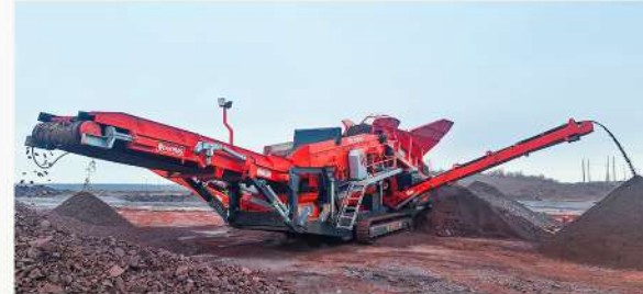
PROVIDES 3 DIFFERENT END-PRODUCTS WITH PRECISE DIMENSIONS BY 2-DECK SCREEN
